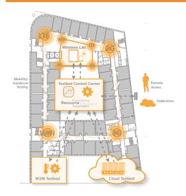
The FUSECO Playground is an open and independent laboratory for network operators, equipment manufacturers, application developers, integrators and applied research organizations. It enables hands-on testing and validation of Cloud, M2M, fixed and mobile Broadband applications, systems and protocols.
